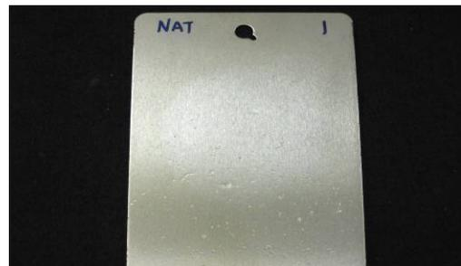
Although one can quite clearly see the disc where the molded rubber has been in contact with the panel, there is no visible difference in the surface appearance of the two panels. The anti-moisture barrier has, indeed, been very effective in preventing the two things that cause corrosion, oxygen and moisture, from attacking the metal surface.
