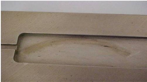
The degree of fouling is much less extreme, mainly because the release system employed has enough barrier property to prevent large-scale re-deposition of the bonding agent on the mold surface.
