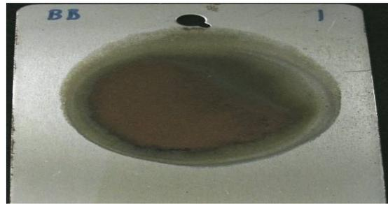
After exposure, there is only minor corrosion in the land areas of the panel, but most noticeably, the area where the disc has been molded has turned a rusty red color. This is a clear indication that even an anti-moisture barrier cannot totally isolate the metal from atmospheric oxygen and moisture
